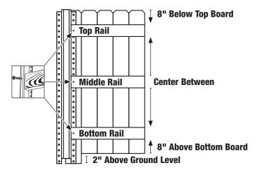
**NOTE:** if the ground slopes, be sure to cut both rail-ends diagonally to allow a flush fit against the rail pocket of the hat section.
