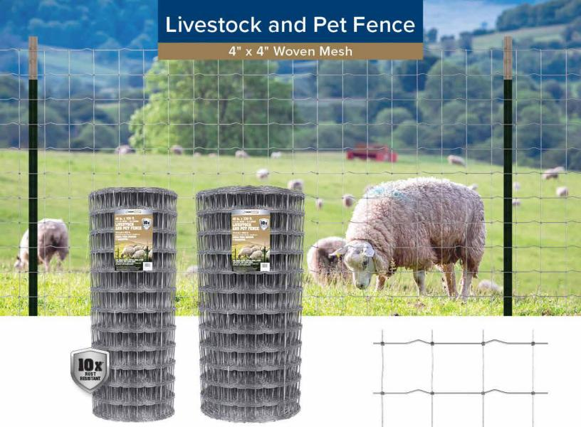
The proprietary production process of FarmGard® livestock and pet fence features 10x corrosion protection\*. Our livestock and pet fence is made of Class 1 zinc coated steel wire. Top and bottom line wires are made from 10 gauge wire with 12.5 gauge filler wire in between. This fence features a 4" x 4" woven mesh design. These fences are built to last and resist buckling or sagging. Meets or exceeds ASTM A116-11.
